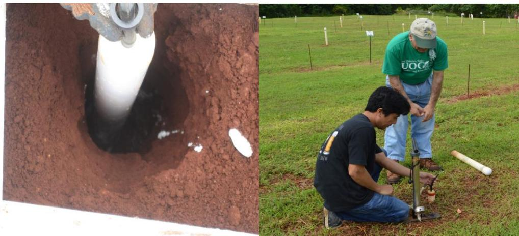
Figure 1: Preparation & Setup of subsurface Lysimeters
