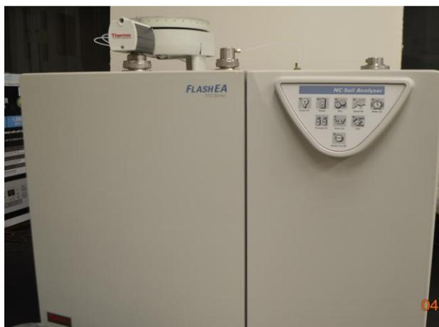
Figure 4: Nitrogen and carbon analyzer (FlashEA 1112 Series) that was used for soil and compost analyses
