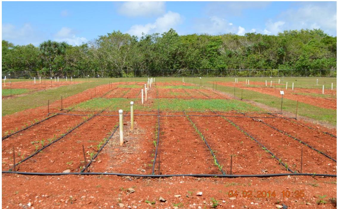
Figure 7: Drip lines (8) with 20 drip emitters per row at 30.5 cm intervals (1 ft.)
