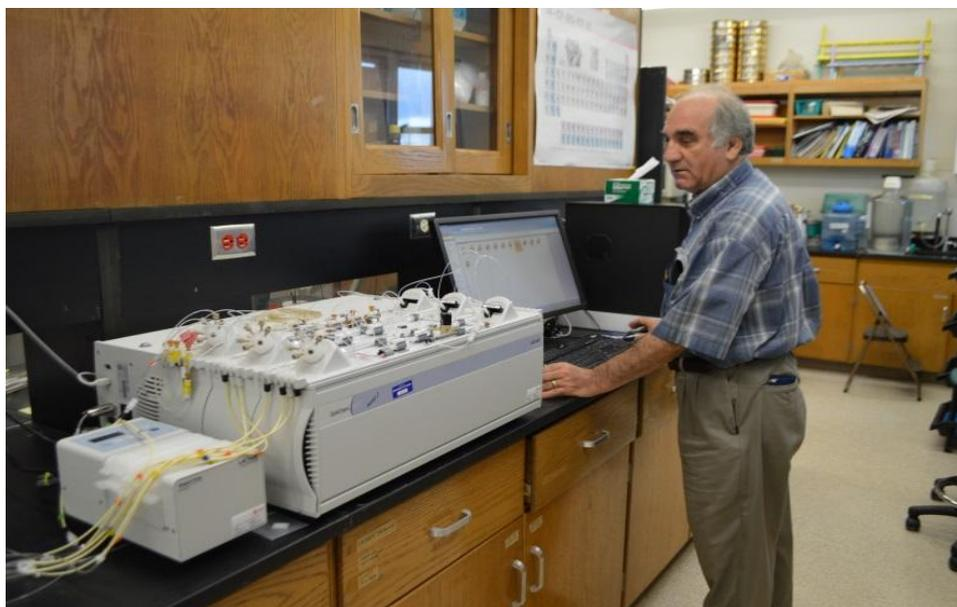
Figure 3: Flow Injection Analyzer (FIA)(QuickChem 8500 Series 2 model) for nitrate ( $\text{NO}_3^-$ ) and phosphate ( $\text{PO}_4^{3-}$ ) analyses
